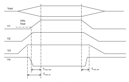
Figure 4: Output Voltage Timing
